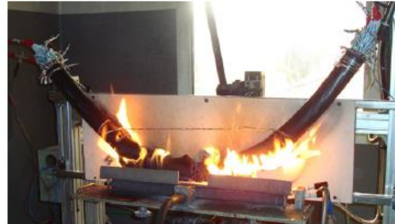
Fire with mechanical shock IEC 60331
